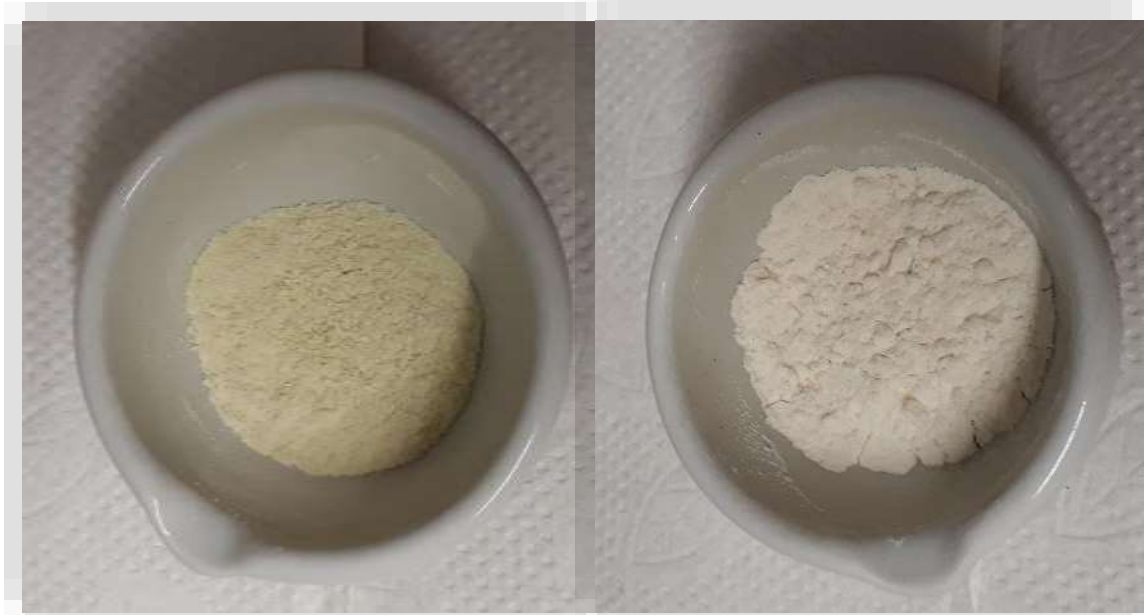
Figure B 5. Freeze-dried green banana flour (left) and wheat flour (right)
