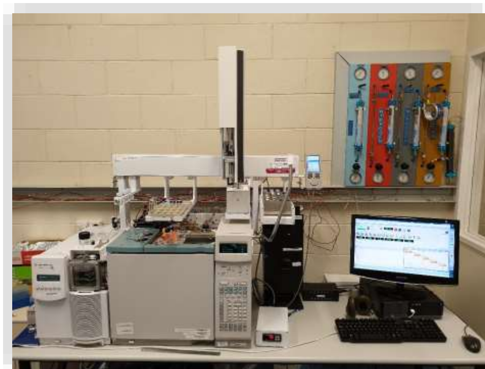
Figure 8.2. Gas chromatography mass spectrometry setup
