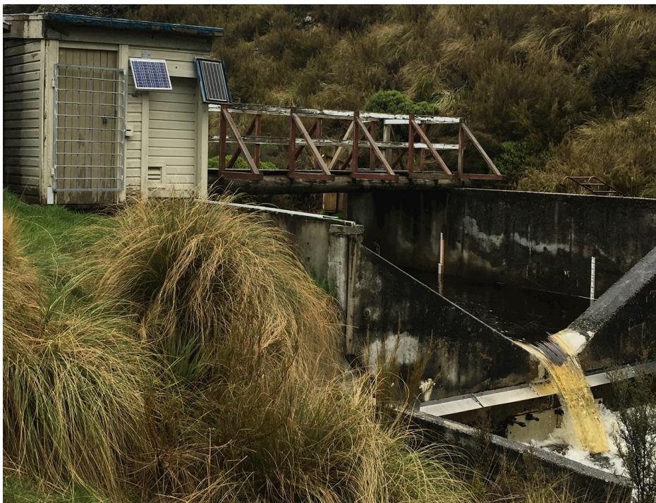
Figure 3.9 Streamflow through the v-notch weir draining the Glendhu experimental tussock catchment (GH1). The water shows a distinct yellow hue that is frequently observed in both GH1 and GH2 catchments.
