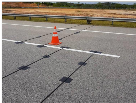
Figure 2. Pneumatic tubes laid across the traffic lanes.
