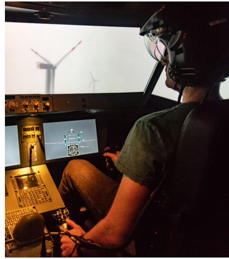
(b) Study II – Pilot wearing the JEDEYE™ see-through HWD in the GECO simulator.
