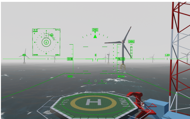
Figure 5 – The pilot’s view during the landing maneuver with the superimposed symbology generated by the monochrome green JEDEYE™ helmet. The symbol set comprises a head-up PFD (center of the image), DLR’s visual conformal landing symbology (lower center), and the developed VCI-OAWD (upper left).
