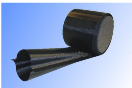
Figure 1 DLR's coilable carbon composite mast during coiling/uncoiling
