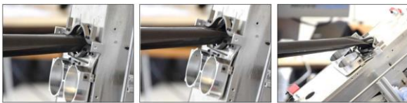
Figure 3 Boom failing at the spot it leaves the GOSSAMER-1 deployment mechanism during sail tensioning limit load tests.
