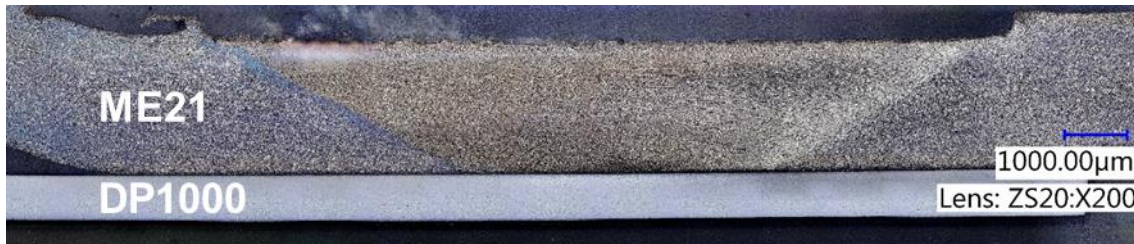
Fig. 11: FSW ME21-DP1000 lap joint: Cross section.
