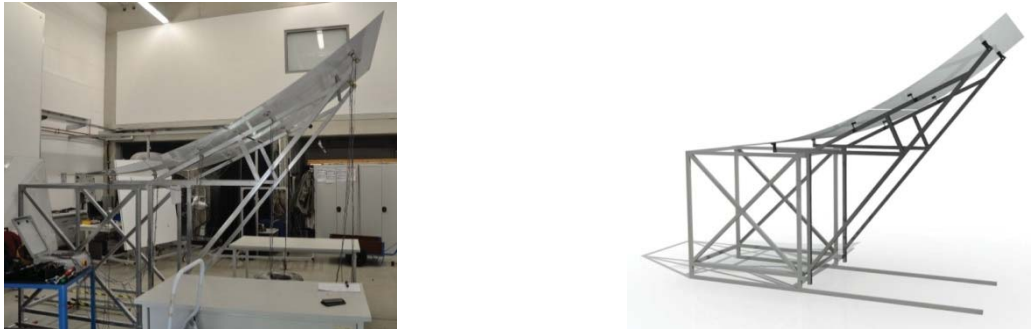
FIGURE 4. Real and CAD image of the laboratory structure employed for the performed deflectometry measurements of RP3 mirrors and the subsequent photogrammetry measurements of the glass brackets
