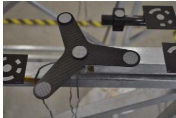
FIGURE 5. Orientation measurement adapter (OMA) for determining the position and angular orientation of the L- and Z-brackets used for mounting mirrors of RP3 geometry in EuroTrough collectors
