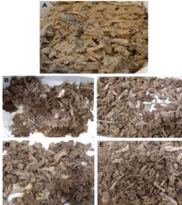
Figure 8: Appearance of samples of FSs during the process of drying at 40°C with and without air-circulation. A. Wet FSs at zero time point, B and C. FSs dried with air-circulation after 26 and 47 hours; D and E. FSs dried without air-circulation after 27 and 51 hours.
