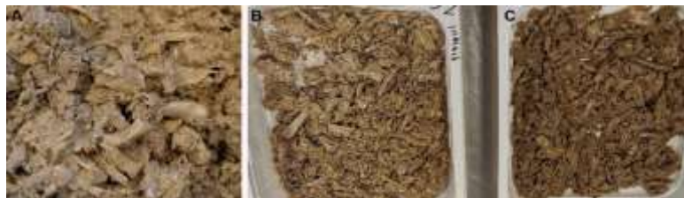
Picture 7: Appearance of samples of fish sediments (FSs) at the final point of drying (450 hours) at 25°C with and without air-circulation. A. Wet FSs, B. FSs dried with air-circulation; C. FSs dried without air-circulation. Photos presented in B and C: Ola Ween.
