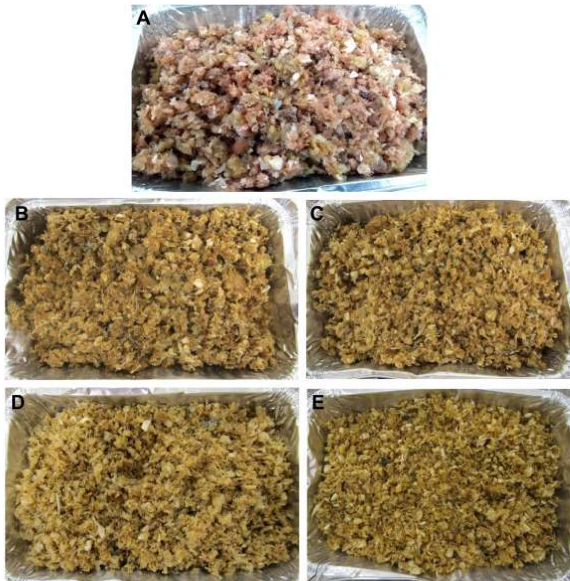
Picture 11. Appearance of samples of minced fish backs (MFBs) at different time points during the drying process in a drying cabinet at 25°C with air-circulation. A. Wet MFBs at zero time point, B. MFBs after 24 hours of drying, C. MFBs after 29 hours of drying, D. MFBs after 48 hours of drying, E. MFBs after 99 hours of drying.
