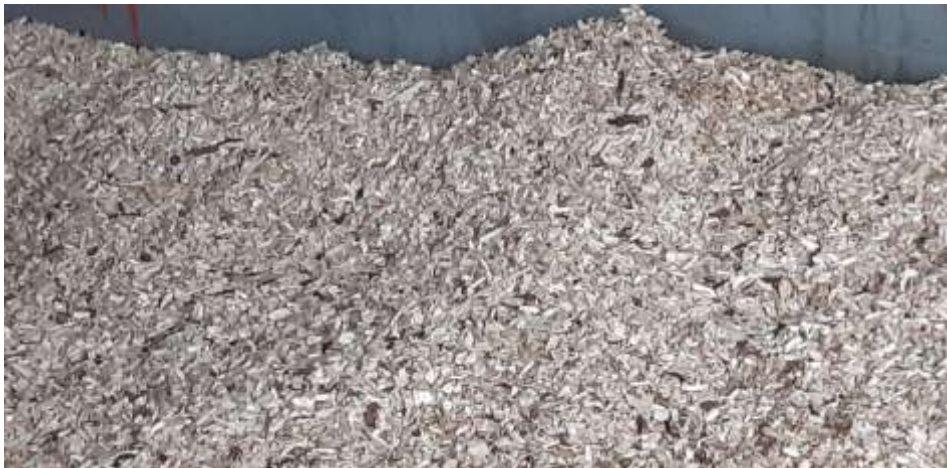
Picture 4: Forest chips that are used in the Tingvoll Flis og Varme AS combustion plant, Tingvoll Farm. Photo: Ingvar Kvande.
