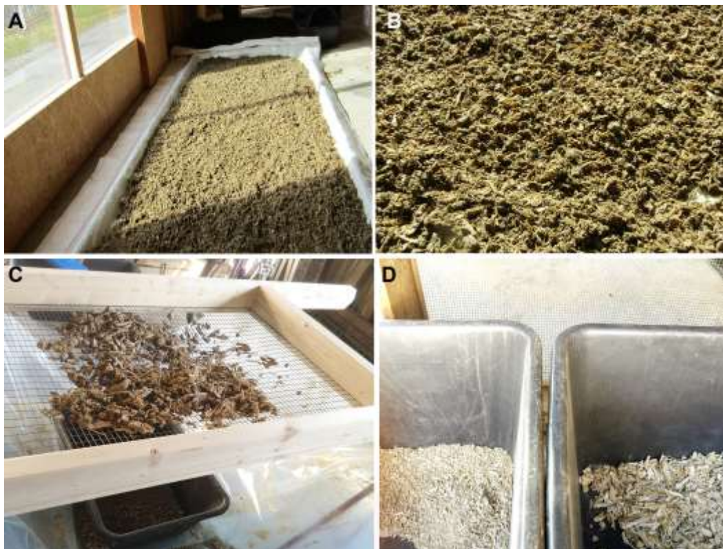
Picture 6: Drying and sieving of FSs. (A) Drying of FSs on a plastic sheet in a room, (B) A closer view of FSs during the period of drying, (C) Sieving of dried FSs, (D) FSs with small size bones and other material (left side) and FS with big size bones and other material (right side). Photos shown in C and D are taken by Anne de Boer.
