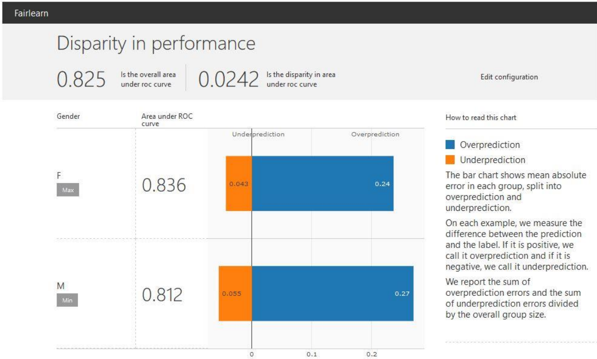
Figure 35: Example dashboard of fairlearn toolkit for gender-based bias analysis of Mean model performance disparity on 10,000 random sampled student predictions
