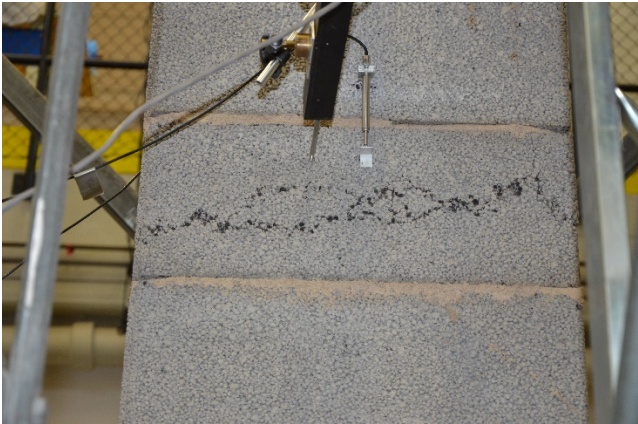
Figure LWA2_W7_1 Flexural compressive failure at mid-height of the wall.
