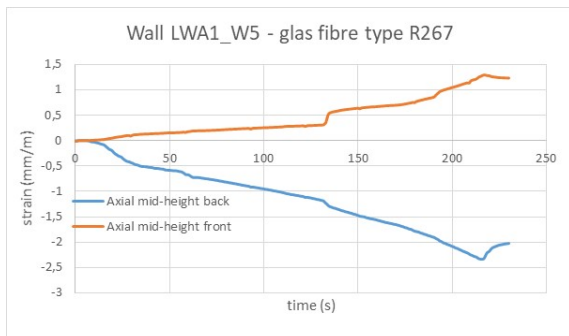
Figure LWA1_W5_3 Axial strains at mid-height vs. time – front (tension) and back (compression) side.
