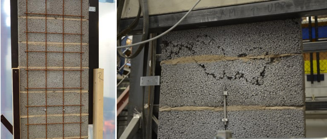
Figure LWA1_W1_1 Mesh reinforcement (left); Crushing below the load application plate (right).
