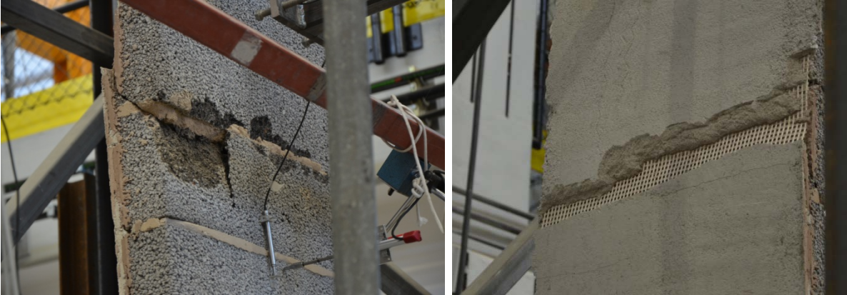
Figure LWA1_W6_1 Flexural compressive failure
