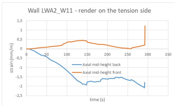
Figure LWA2_W12_3 Axial strains at mid-height vs. time – front (tension) and back (compression) side.
