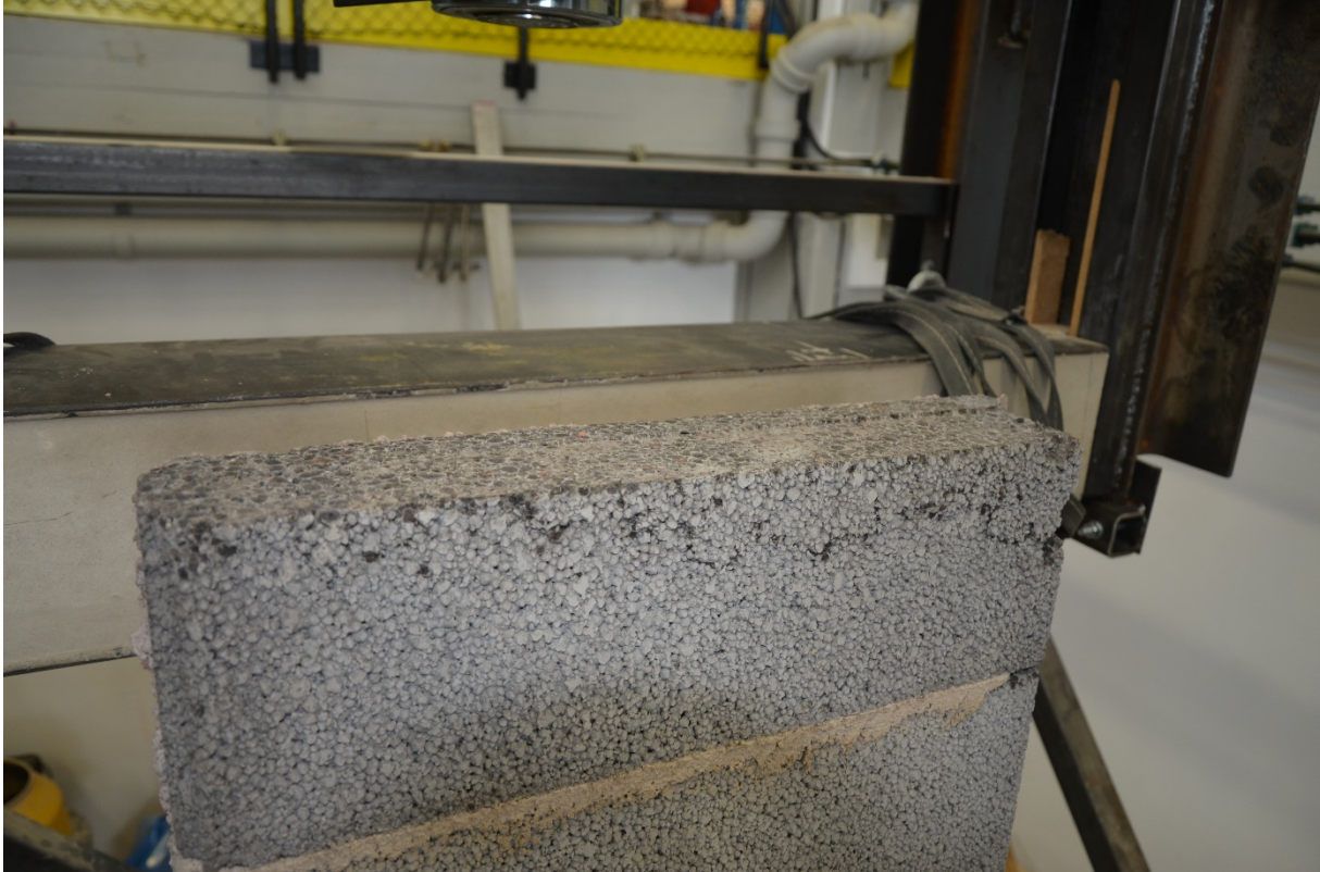
Figure LWA2_W4_1 Crushing at the load application plate.
