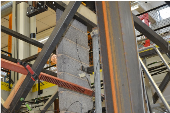
Figure LWA2_W1_1 Flexural compressive failure at 2/3-height of the wall.
