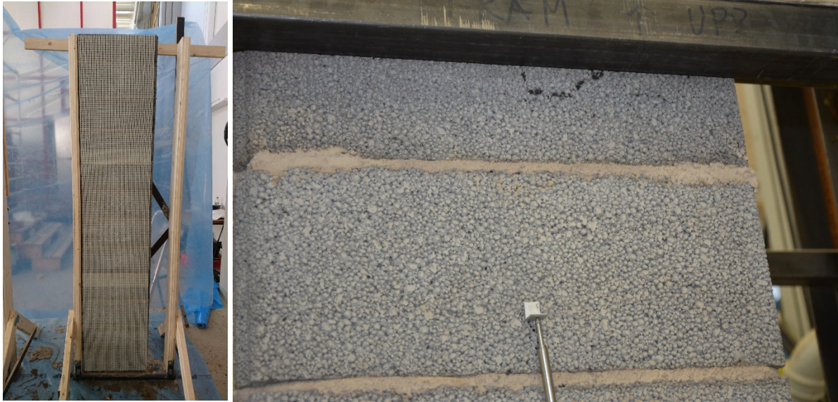
Figure LWA2_W3_1 Glass fibre mesh attached directly to the surface of the wall (left); Local crushing at the upper loading plate (right).
