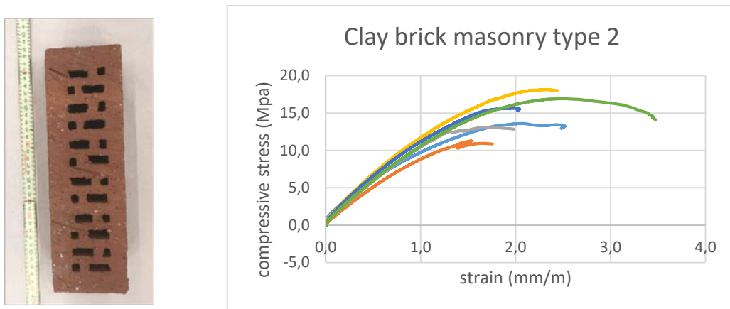
Figure 2.2 Clay brick masonry type 2. Perforated bricks (left); stress – strain relationship (right).
