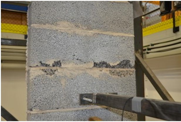
Figure LWA1_W5_1 Flexural compressive failure at 2/3-height of the wall.
