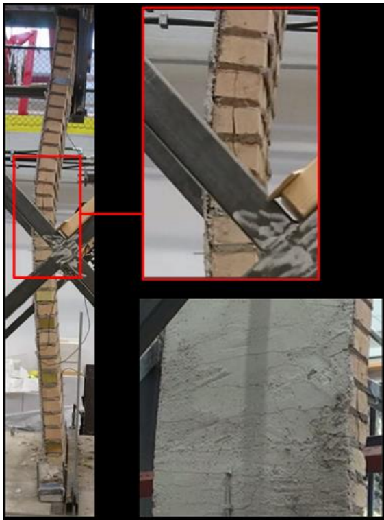
Figure B1_W6_3 Flexural compressive failure at mid-height of the wall (left and upper right); Crack pattern before failure (lower right).
