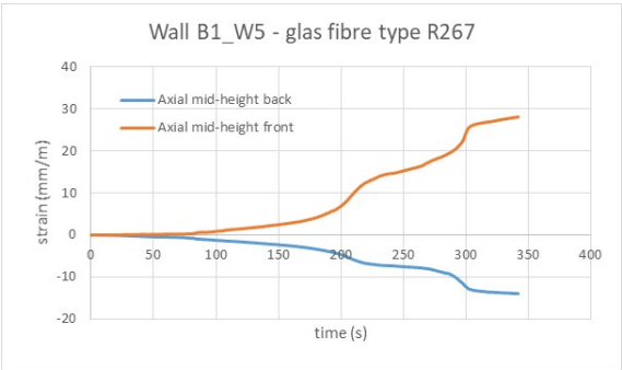
Figure B1_W5_2 Axial strains at mid-height vs. time – front (tension) and back (compression) side.
