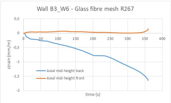
Figure B3_W6_3 Axial strains at mid-height vs. time – front (tension) and back (compression) side.
