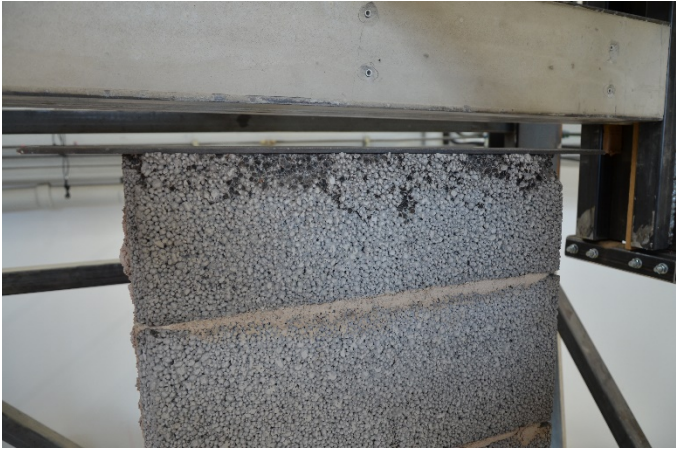
Figure LWA2_W6_1 Local crushing at the upper loading plate.
