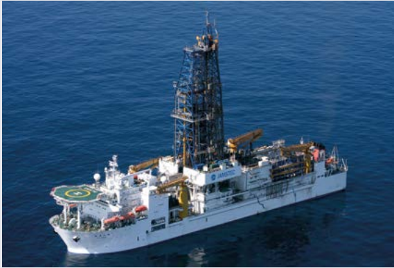
IODP's Chikyu scientific drilling vessel operated by the Japan Agency for Marine-Earth Science and Technology (JAMSTEC). The D/V Chikyu is currently the world's most advanced scientific drilling vessel, capable of drilling deeper below the seafloor than any other science drilling vessel to date. (photo: JAMSTEC/IODP)
