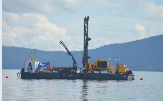
ICDP's Deep Lake Drilling System (DLDS), a barge and drill rig combination to recover unconsolidated sediment and hard rock cores from deep lake bottoms. The system is capable of recovering core from up to 1,400 m depth. Shown here is the DLDS in action on Lake Towuti (2° S, 121° E), Indonesia, anchored at a water depth of 150 m recovering 175 m of sediment core and the underlying bedrock. (photo: Marina Morlock)
