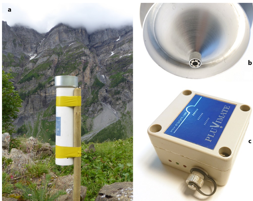
640 Figure 4. Drop-counting rain gauge used for rainfall measures. The Pluvimate is set-up vertically between 0.8 and 1.2 meters above the ground level (a). A tip at the end of the funnel (b) creates a calibrated drop of water that falls on the sensor, (c) which counts and records the number of drops during a given amount of time.
