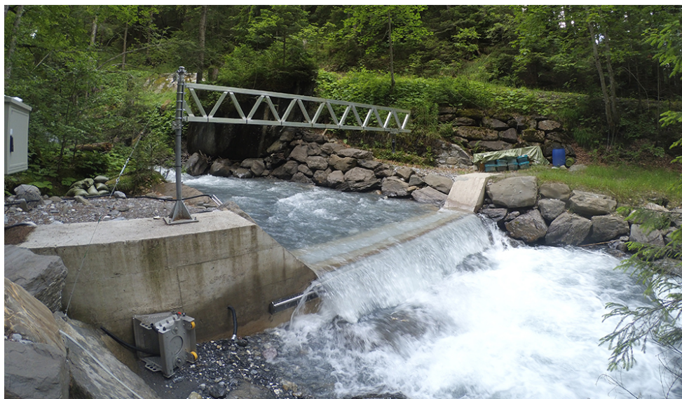
Figure 2. River stage measure at the outlet. The streamflow is here measured between 0.96 and 1.13 \text{ m}^3 \cdot \text{s}^{-1} .
