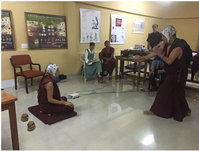
Fig. 2 Example of the EEG setup. One challenger (standing) and one defender (seated) are both wired with an EEG cap. Another monastic is seated behind a computer and presses trigger buttons to create events in the EEG data. Video is also collected of each debate, which was subsequently analyzed with behavioral coding software
