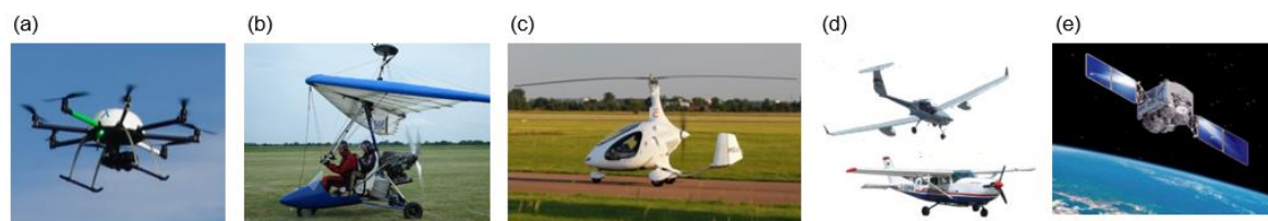
Figure 3. Different air- and spaceborne remote sensing platforms for assessing geodiversity and geotraits, (a) unmanned aerial vehicles (UAV, or drone), (b) micro-light-gravity-controlled (c) gyrocopter-micro-light helicopter, (d, top) Ecodemona, (d, bottom) Cessna, (e) satellite.
