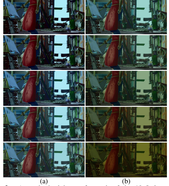
Fig. 3. A synthesised image for each of the 10 Jerlov water types [24] for a scene at depth 1.30m under the water surface, and with the farthest object at 1.65m from the camera. (a) Oceanic water (top to bottom: type I, IA, IB, II, III). Red is the most attenuated, inducing a blue cast. (b) Coastal water (type 1, 3, 5, 7, 9). Blue is the most attenuated, inducing a green cast.
