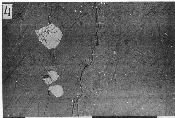
**Figure 4.** Kalimashi Chrome Ore, as mined (BEI). Three different minerals may be noted: chromite (light grey) and olivine (dark grey), both on the left of the photo, and pyroxene (medium grey) on the right. The contact between olivine and pyroxene is clear but quite irregular. The whole sample is affected by fractures. Length of white bar = 1 mm.
