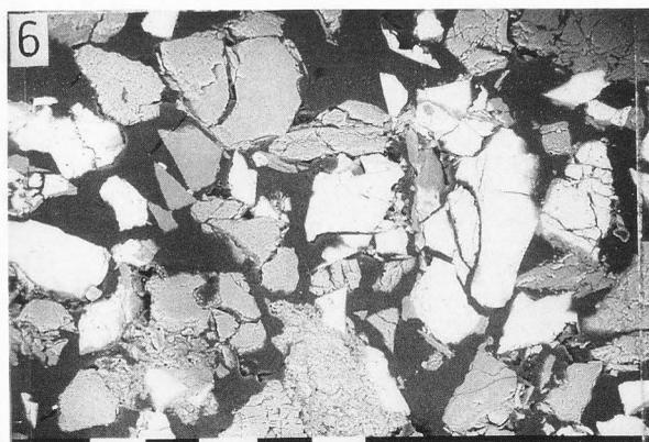
**Figure 6.** Kalimashi Chrome Ore: grain-size fraction between 250 and 500 micrometers after comminution (BEI). Grain texture and composition analysis reveals that marked interpenetration also exists in the comminution products. This sample contains calcite (phase A), which is practically absent in the ore and whose presence, when it can be found, is clearly of secondary origin (water circulation in fractured bodies). Length of white bar = 0.1 mm.
