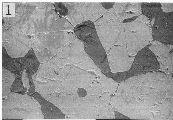
**Figure 1.** Kalimashi Chrome Ore, as mined back-scattered electronic image (BEI). The variability of textural characteristics is evident. Chromite is present both as patches of variable shapes and sizes and as idiomorphs. Fractures occur throughout the whole sample; these are filled with serpentine (chrysotile and microantigorite types). This situation is indicative of the tectonic movements that have affected the ore body. Length of white bar = 1 mm.
