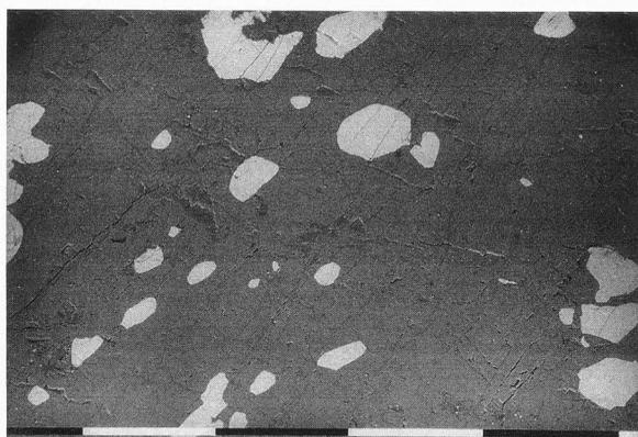
**Figure 3.** Kalimashi Chrome Ore, as mined (BEI). Chromite (light grey) is disseminated in the olivine (medium grey). Chromite is present as both, regular and irregular, particles. It is often affected by microfracture systems filled with serpentine. Length of white bar = 1 mm.
