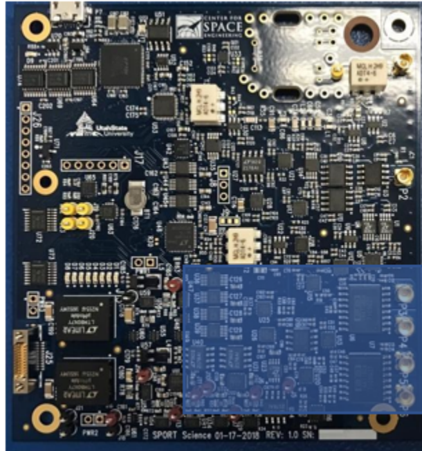
Fig. 4.2: Location of EFP analog components on the USU SWP PCBA
