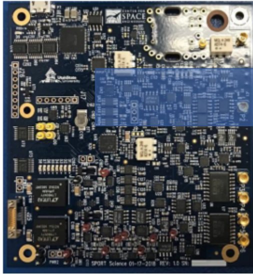
Fig. 3.2: Location of SLP analog components on the USU SWP PCBA
