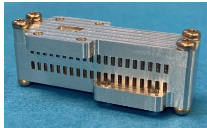
Double-sided groove-gap waveguide.
