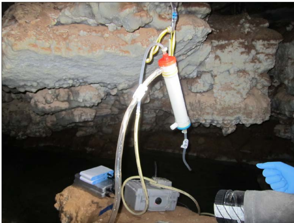
Figure 2. A peristaltic pump being used to collect a water sample in Wind Cave.
