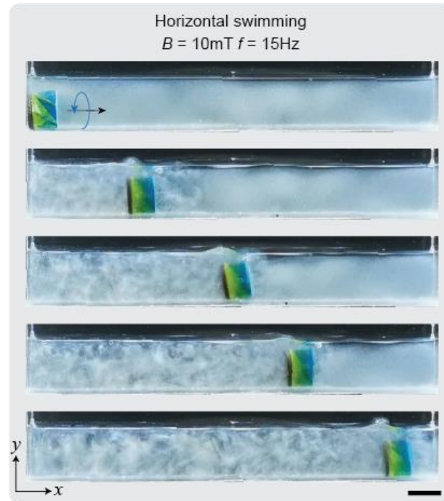
Figure 17 Magnetic Kresling robot swims in the horizontal direction (scaler bar: 13mm)
