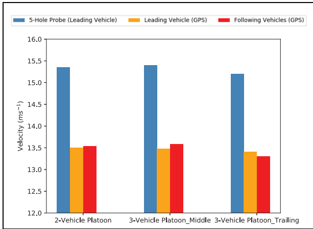
Figure 6. Comparison between the velocity measured using a five-hole probe against the true velocity of the vehicle measured using a GPS.
