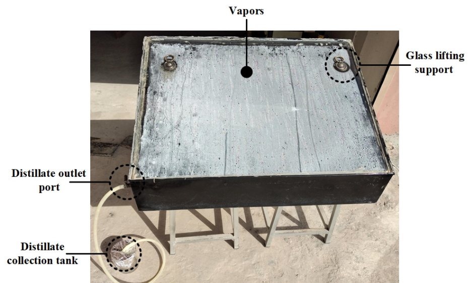
Figure 3. Single slope solar still experimental setup.
