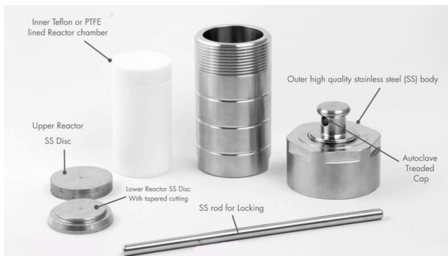
Figure 1.10. Disassembled autoclave reactor.
