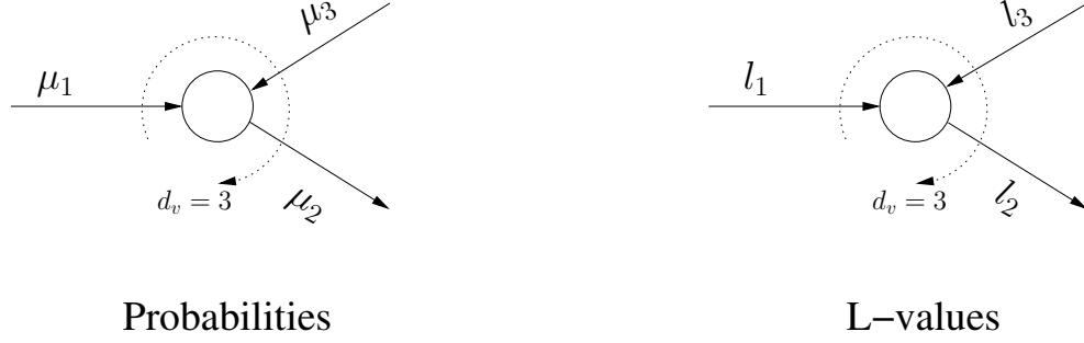
Figure 4.5: Variable node having degree ( d_v ) 3, the outgoing extrinsic message is \mu_2 ( l_2 ) and the two incoming messages are \mu_1 ( l_1 ) and \mu_3 ( l_3 ).
