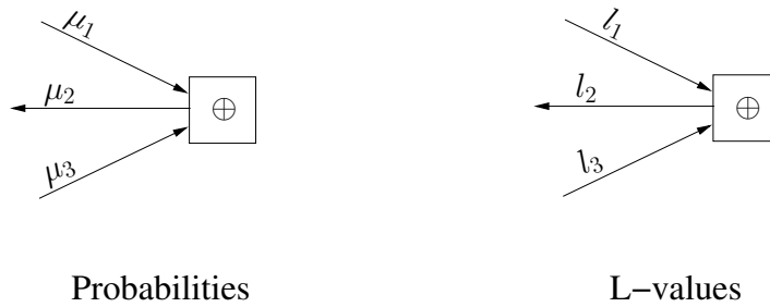
Figure 4.9: Check node having degree ( d_c ) 3, the outgoing extrinsic message is \mu_2 ( l_2 ) and the two incoming messages are \mu_1 ( l_1 ) and \mu_3 ( l_3 ).
