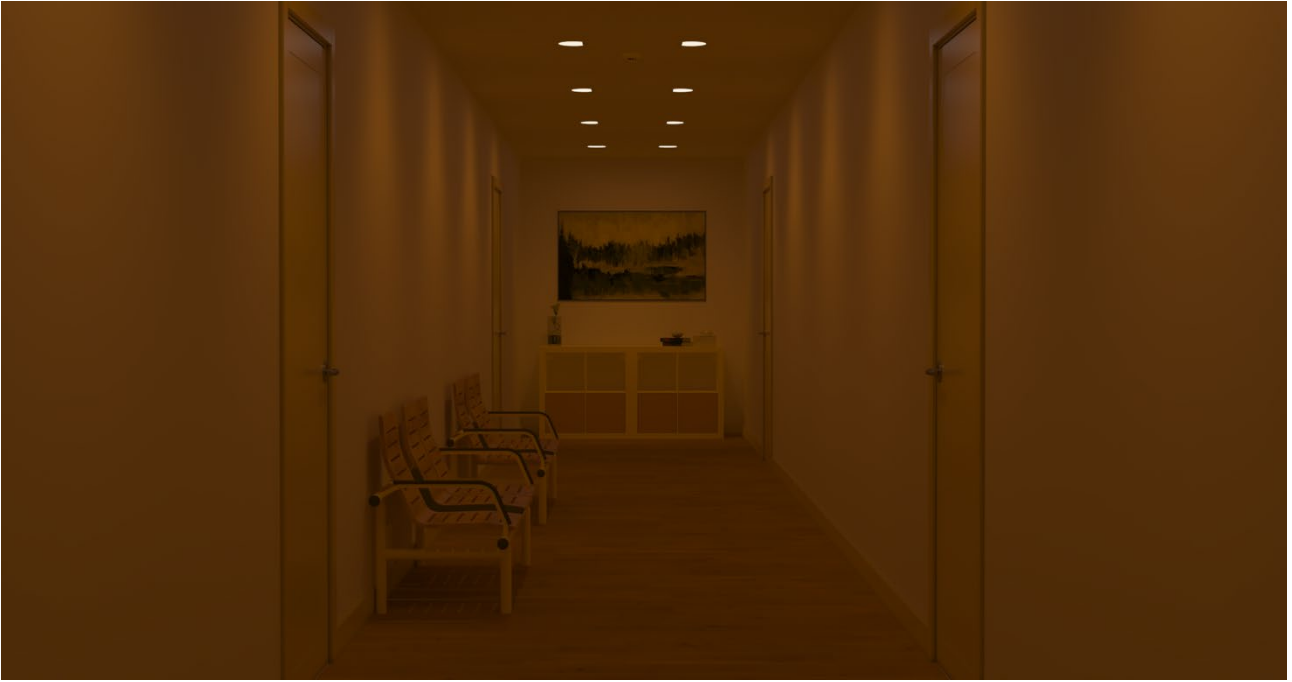
FIGURE 60 Hallway, Wallwasher 20 lux, RSL
