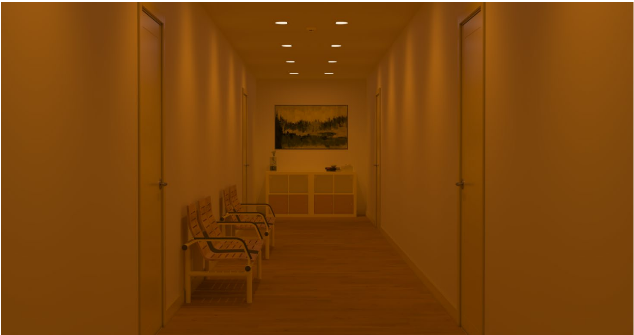
FIGURE 63. Hallway, Wallwasher 50 lux, RSL
