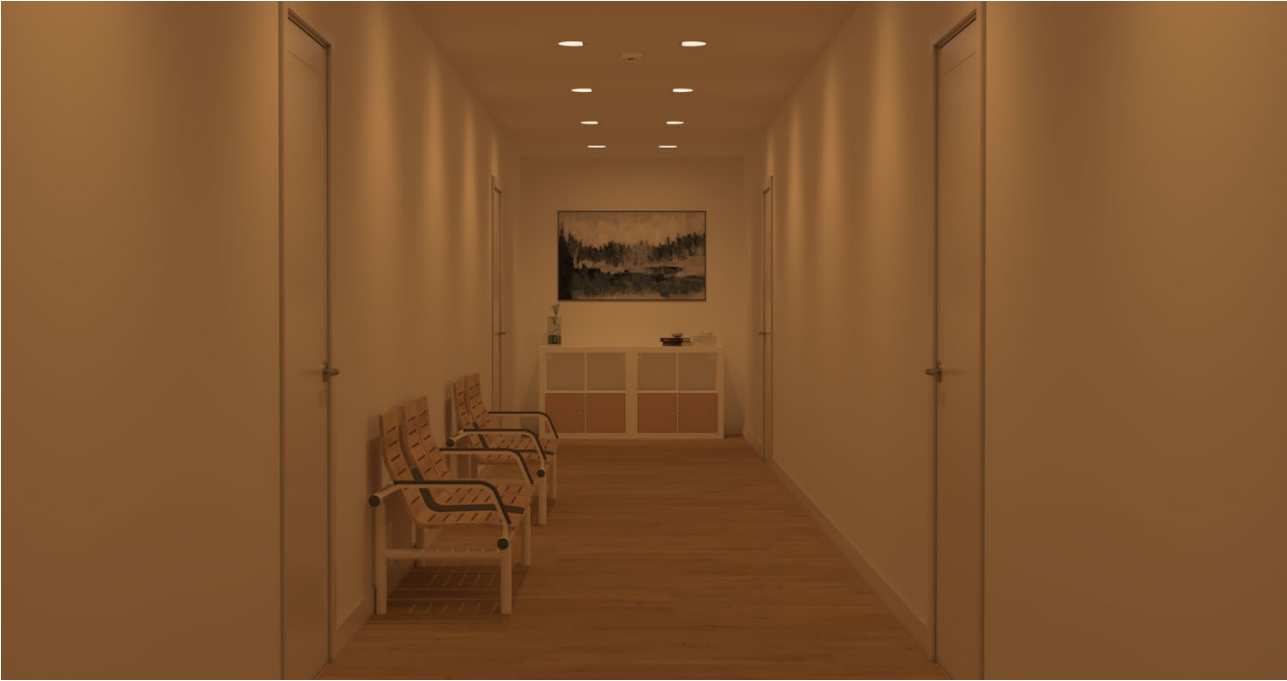
FIGURE 58. Hallway, Wallwasher 70 lux, FSL
