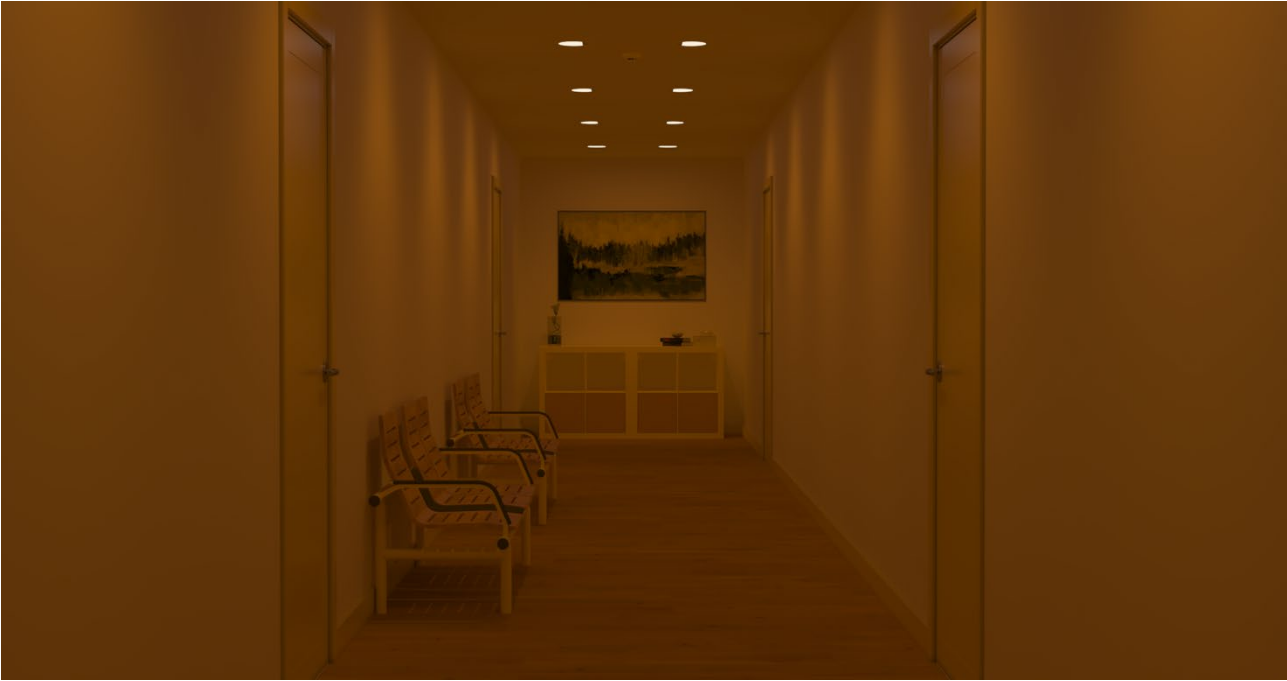
FIGURE 61. Hallway, Wallwasher 30 lux, RSL
