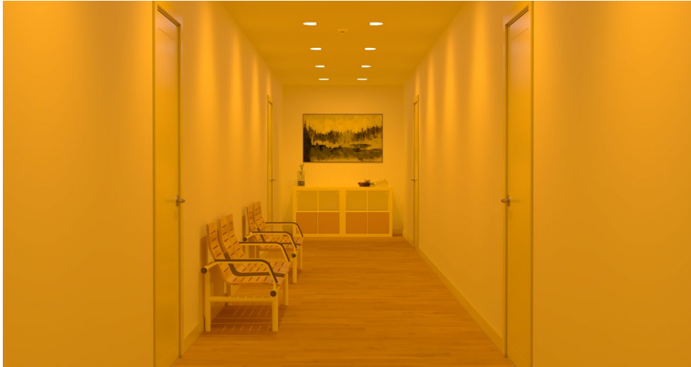
FIGURE 13. One of the visualizations of the hallway – Scenario with wallwashers in RSL providing 50lx average horizontal illuminance on the floor.
