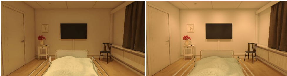
FIGURE 2. A downlight reference scene with the light directly hitting the horizontal plane (left) and a wallwasher scene providing diffuse light reflected from the walls on the horizontal plane (right), under full spectrum lighting (FSL).
