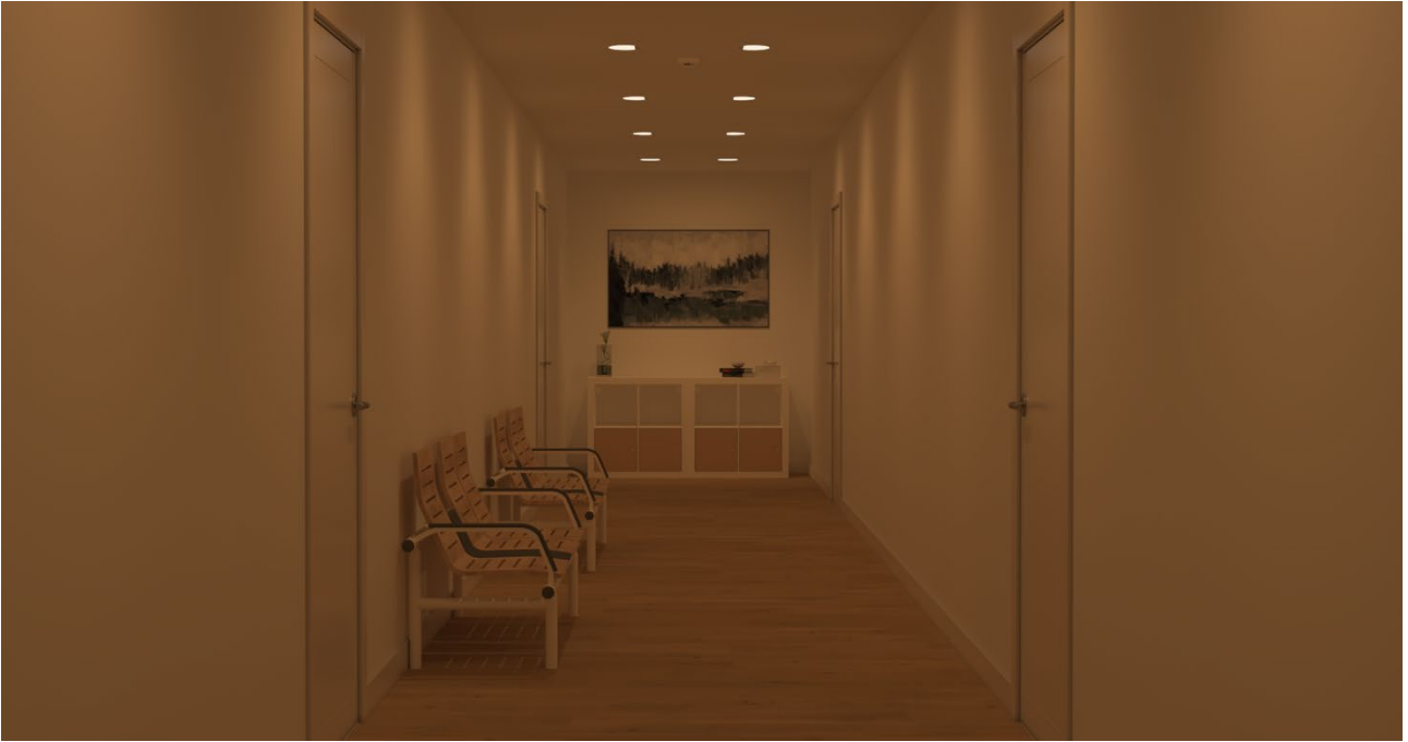
FIGURE 57. Hallway, Wallwasher 60 lux, FSL
