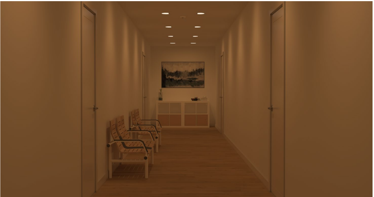
FIGURE 56. Hallway, Wallwasher 50 lux, FSL
