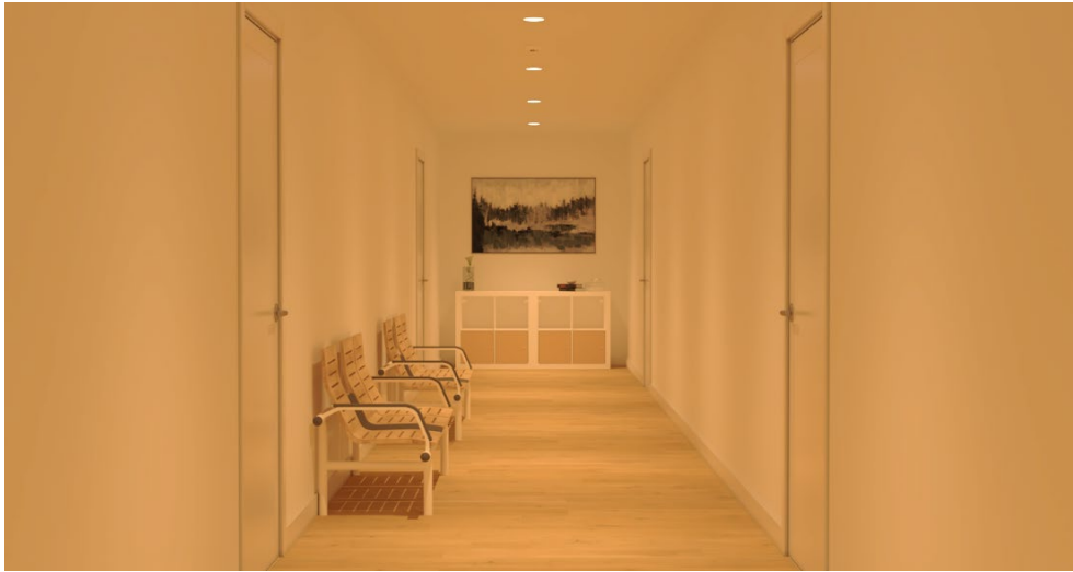
FIGURE 11. One of the visualizations of the hallway – reference scene with downlights in FSL 3000K providing 50lx average horizontal illuminance on the floor.
