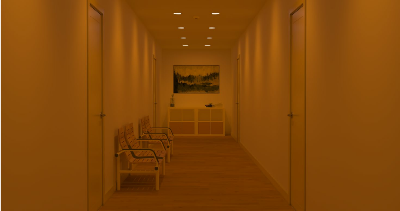
FIGURE 64. Hallway, Wallwasher 60 lux, RSL
