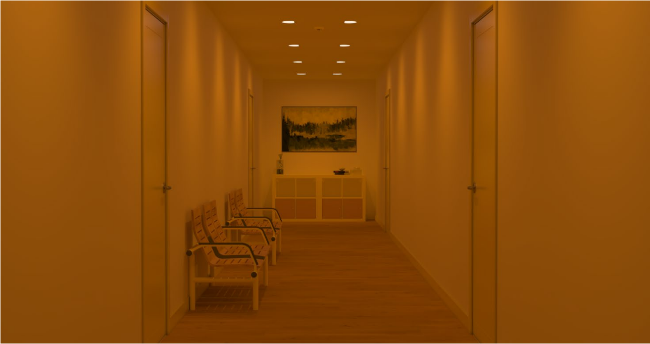
FIGURE 65. Hallway, Wallwasher 70 lux, RSL
