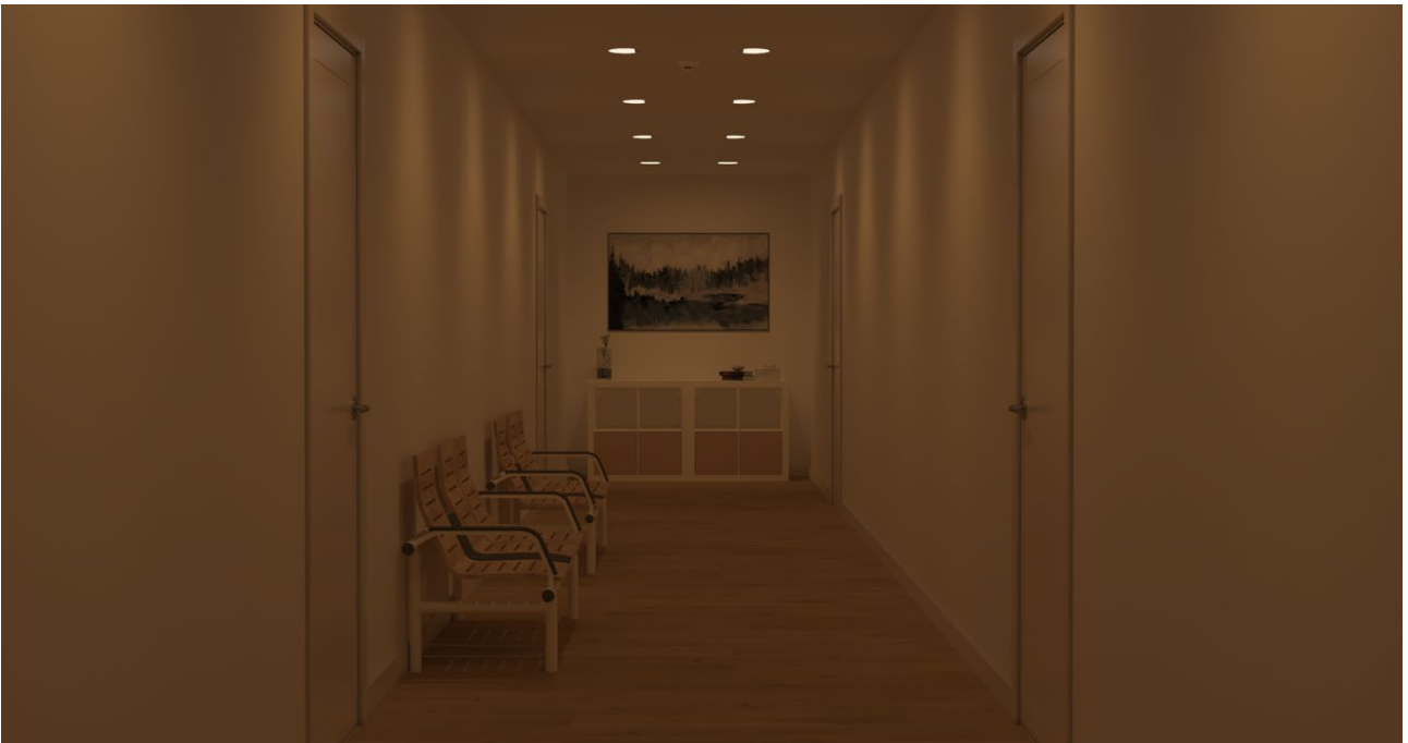
FIGURE 54. Hallway, Wallwasher 30 lux, FSL
