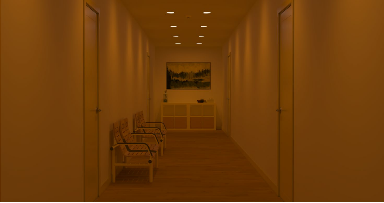
FIGURE 62 Hallway, Wallwasher 40 lux, RSL
