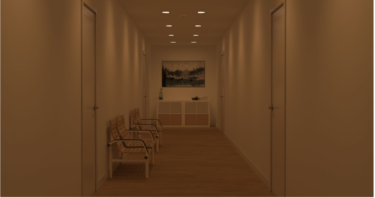
FIGURE 55 Hallway, Wallwasher 40 lux, FSL
