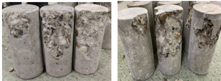
Figure 5. Typical cylinder failures tested at 7 and 28 days.
