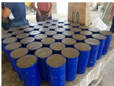
Figure 3. Concrete sample formwork.
