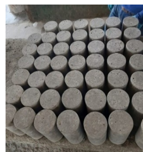
Figure 4. Uncoated concrete cylinders.
