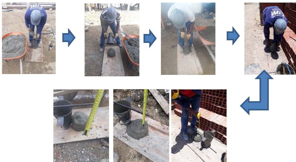
Figure2. Illustration of the settlement test procedure.
