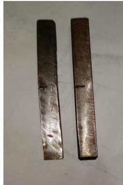
Figure 4. Test specimens tested in the Charpy pendulum impact machine [10].
