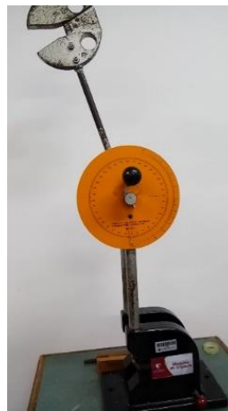
Figure 2. Charpy pendulum impact machine [10].
