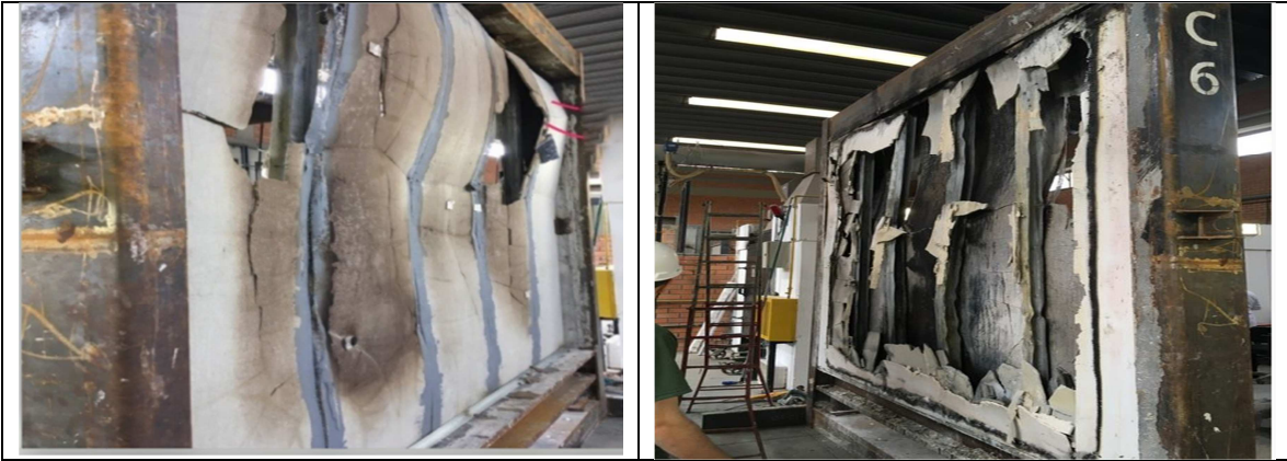
Figure 4. Bubble formation in sample 2, after being tested.
