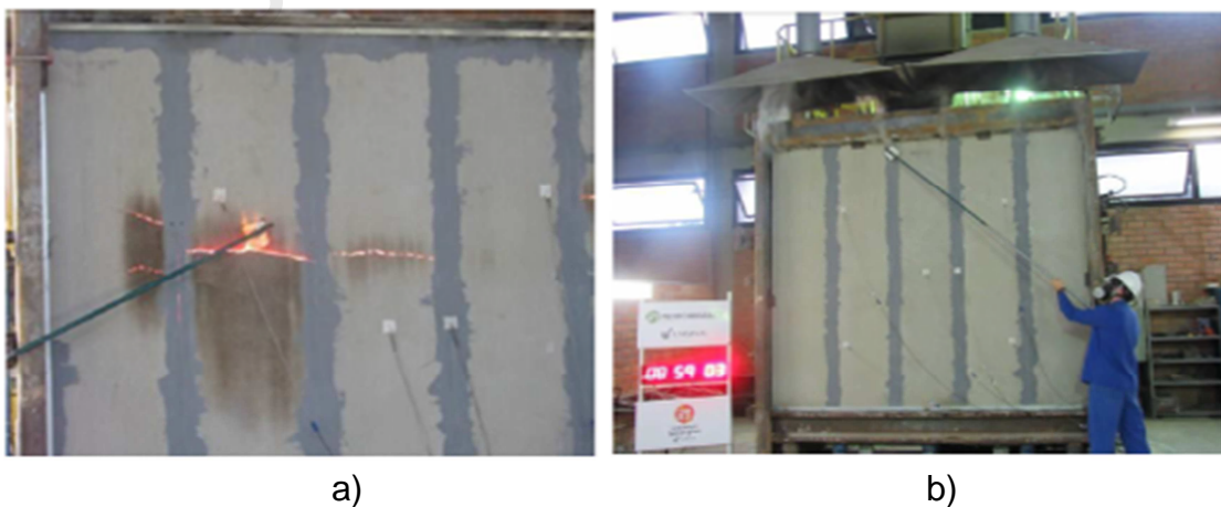
Figure 6. The integrity test procedure for the a) sample 1 and for the b) sample 2.
