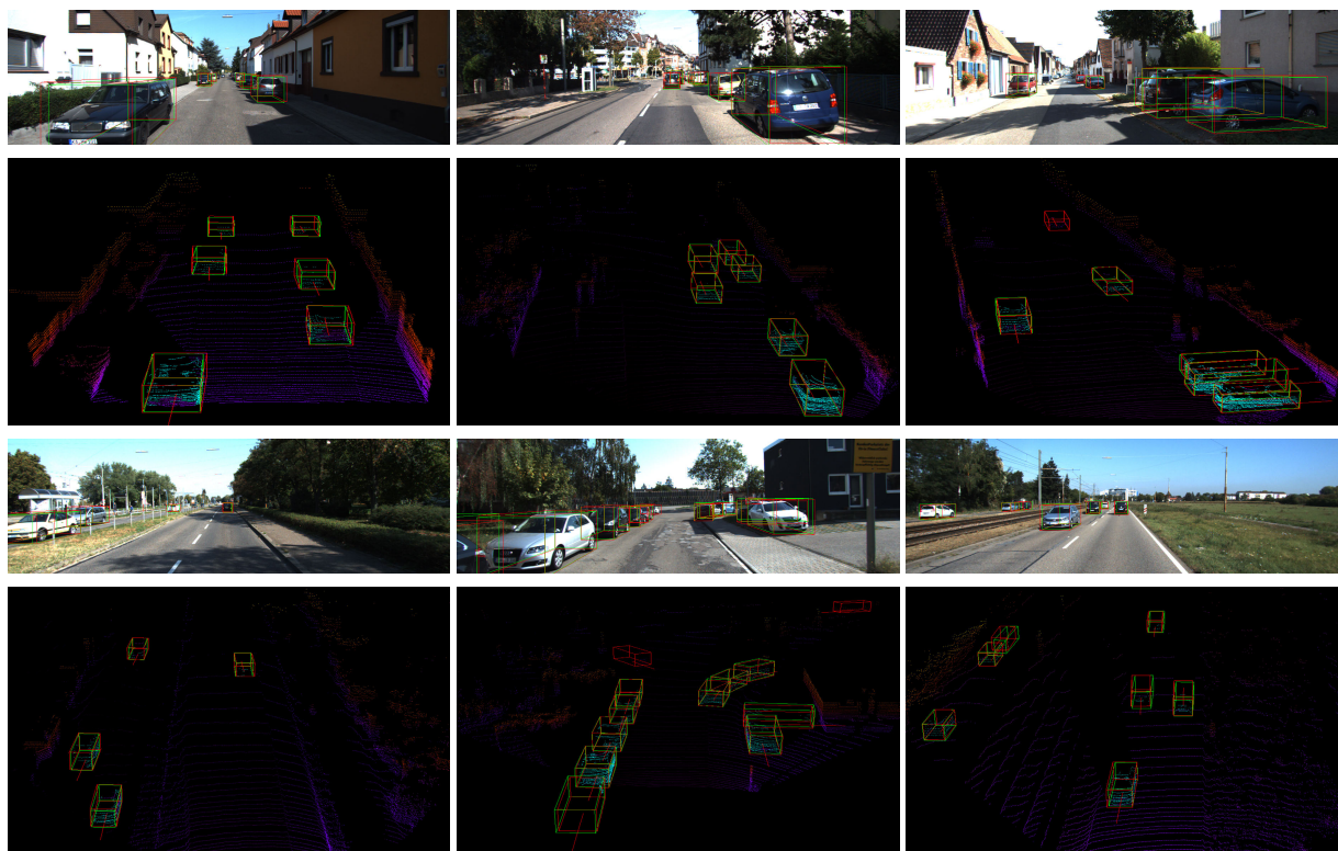
FIGURE 9. Qualitative results on the KITTI validation dataset. The predicted objects and the ground truth objects are shown in red and green bounding boxes respectively. We also project the bounding boxes to the RGB images for better visualization.
