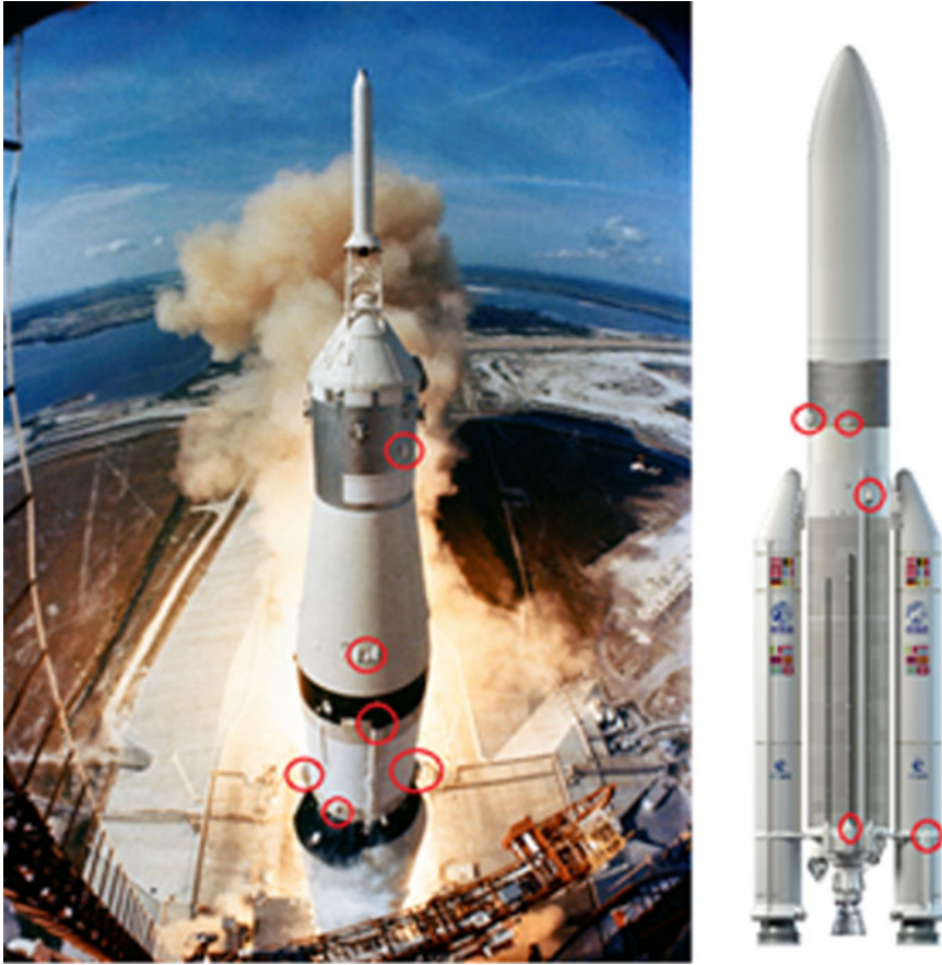
Figure 1. Examples of wedge-like fairings on Saturn V and Ariane V launch vehicles (NASA/ESA).
