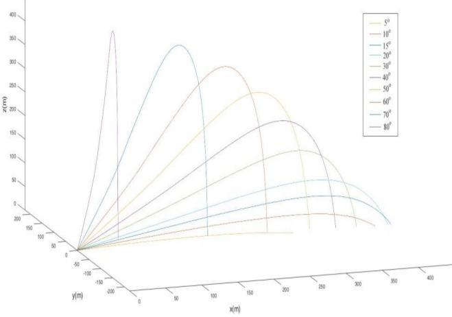
Figure 6. 3D trajectories, plotted in the MatLab, of the fragment (with 7.89g mass) for the different initial elevation angles
