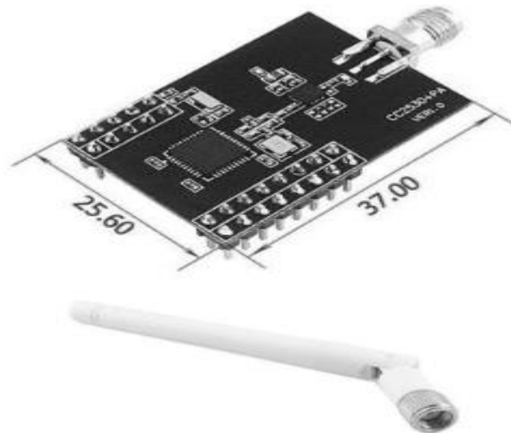
Figure 4. 2.4GHz ZigBee module for sending CNC results wirelessly to remote control panel
