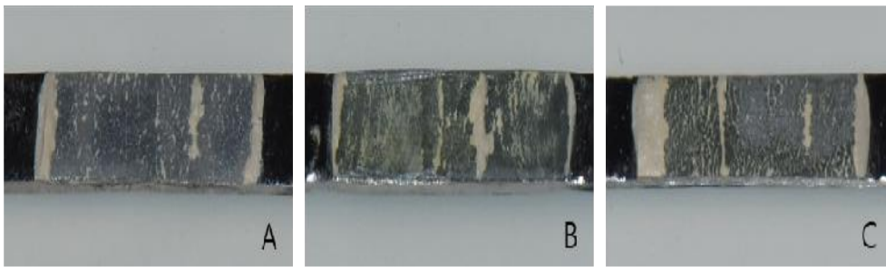
Figure 12. Metal-ceramic failure surface after debonding of the ceramic: (A) casting, (B) milling, and (C) SLM
