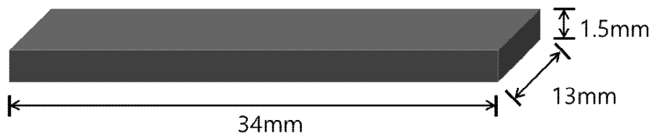
Figure 2. Schematic diagram of the shape of the alloy specimens.
