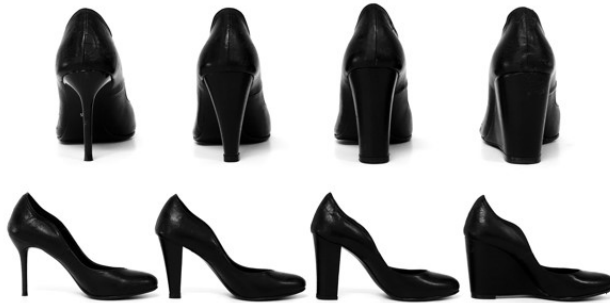
Figure 11: Four manufactured high heels with different heel areas; from left to right, narrow heels (0.9 cm·0.9 cm), moderate heels (1.5 cm·1.7 cm), wide heels (2.8 cm·2.9 cm), and wedge heels (one-piece of the sole and heel).
