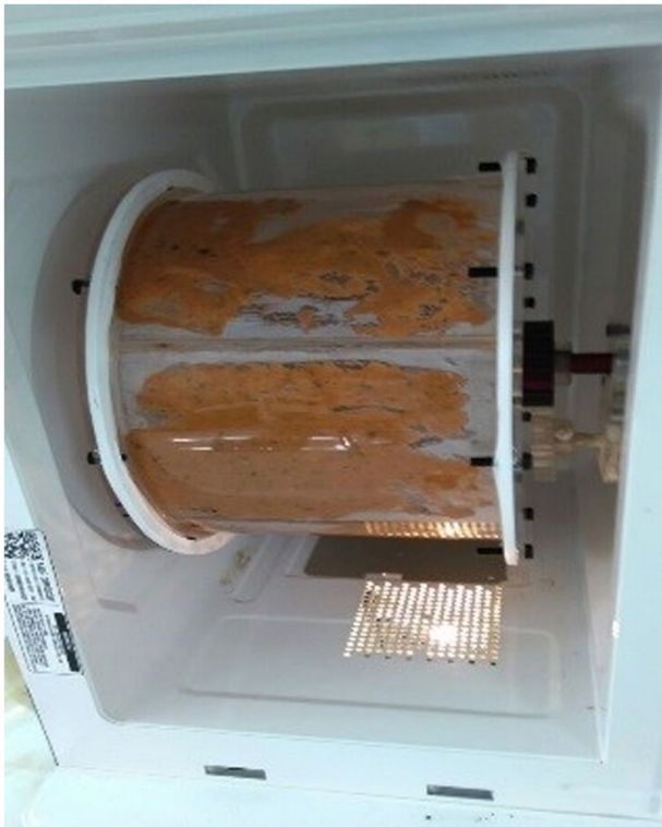
FIGURE 2 Microwave oven with rotary drum used in the drying experiment
