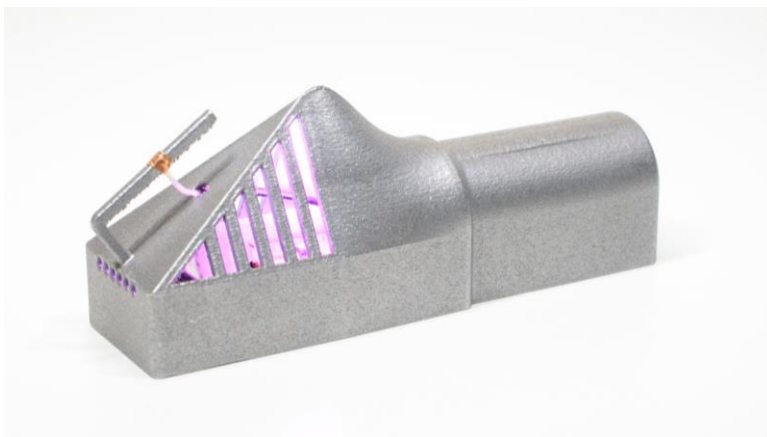
Figure 9. Etteplan's printed demo device with sensors tracking acceleration, temperature, air pressure and air humidity. © 2020 Etteplan.
