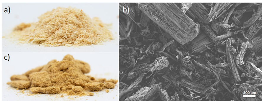
Fig. 4 a Photograph and scanning electron microscopy image of the screened sawdust used in the study. b Photograph of the screened sawdust compressed without IL; compression pressure 10 MPa, temperature 160 °C, and compression time 3 h. c SEM image of the screened sawdust used in the study
