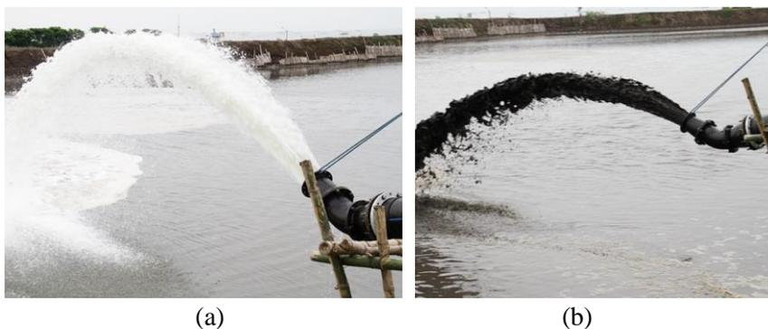
Gambar 4. 6 Kondisi (a) *clear water* (b) *slurry/mud*
