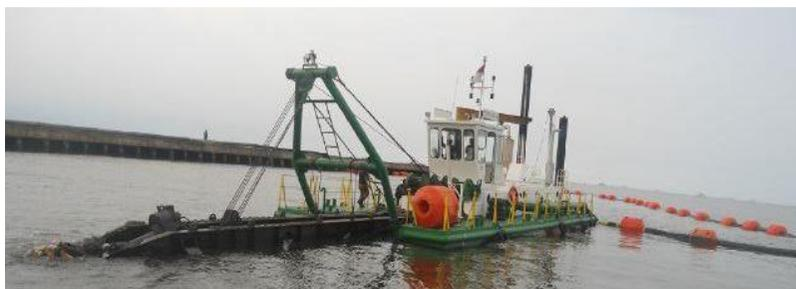
Gambar 2. 5 *Cutter suction dredger*
