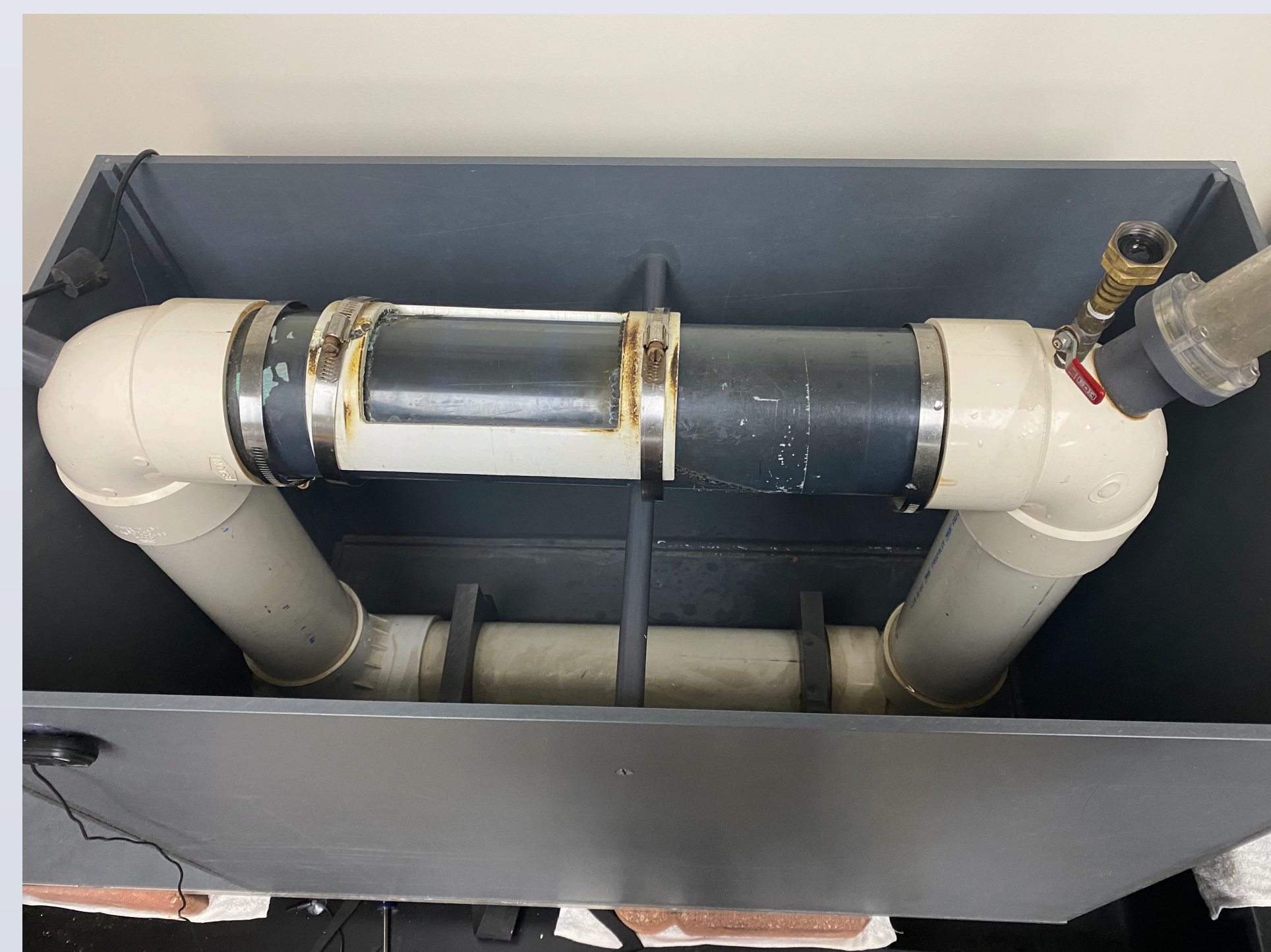
Figure 3: Photo of the flow chamber from the top looking down. Photos taken by Jessica Wilks
