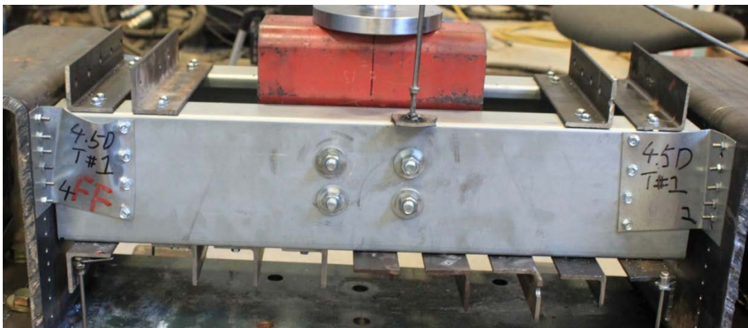
Figure 5.5: Failure mode of joist 4.5D T#1
