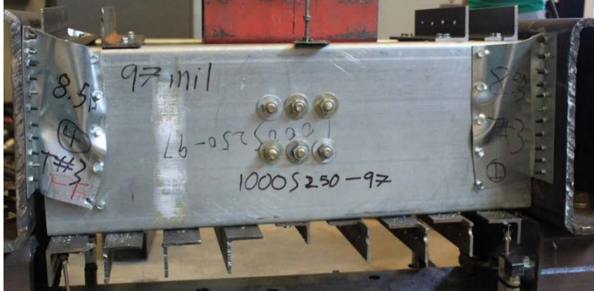
Figure 5.12: Failure mode of 8.5B T#3
