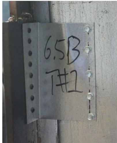
Figure 5.9: Failure mode of shear test II6.5 #1
