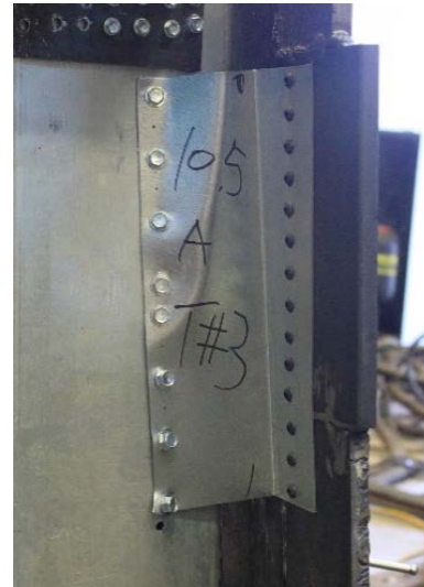
Figure 2.4: Test result of clip angle II10.5 b #1
