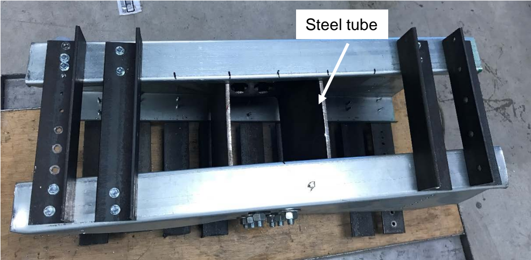
Figure 5.3: Connection details of the two joists (photo taken after test)
