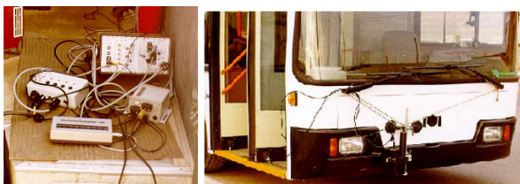
Fig. 8. Measuring tooling Datron and its arrangement on trolleybus
