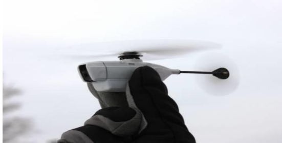
Figure 1.7 Micro UAV (Black Hornet Nano) (Yarrish, 2015)
