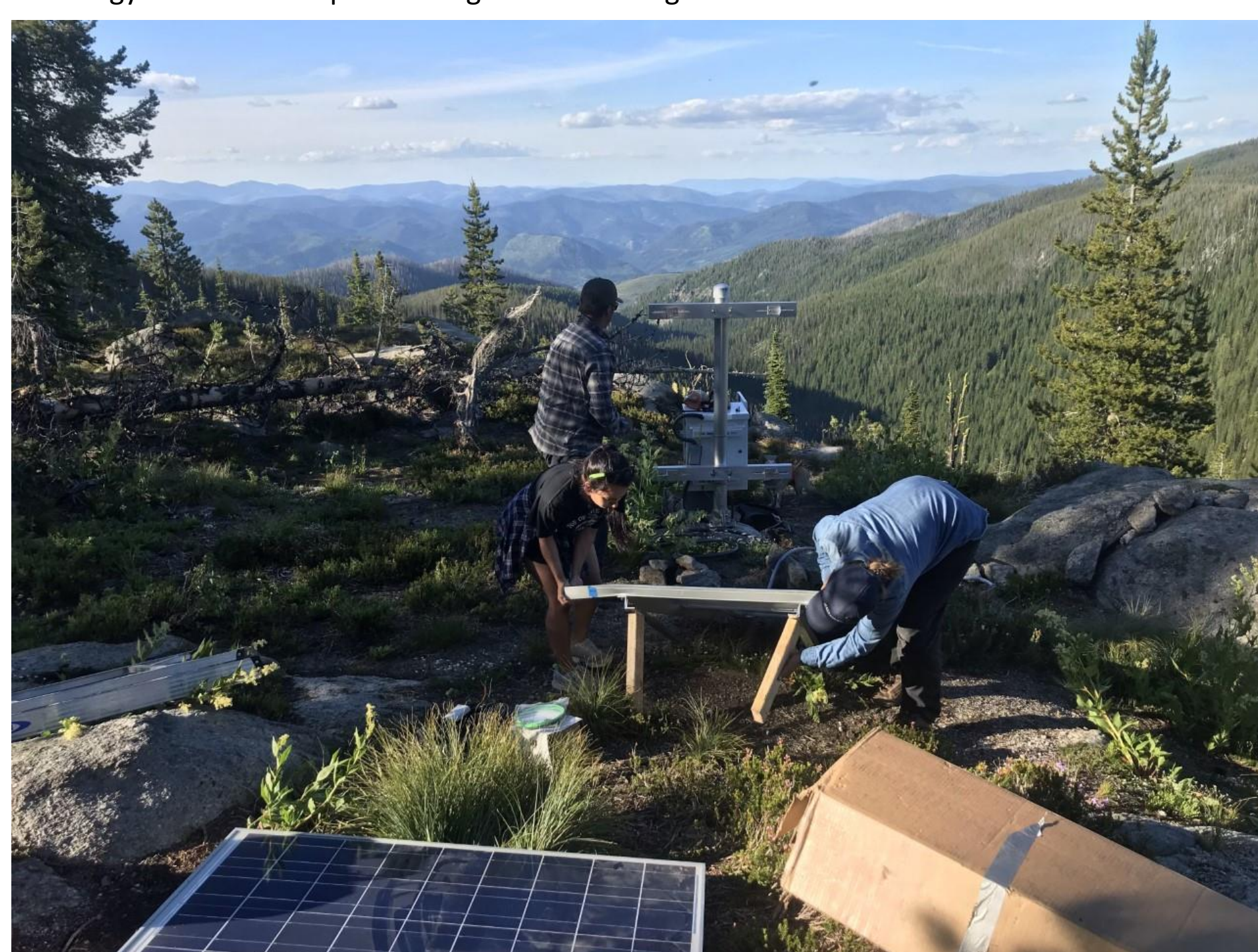
Summer 2020 Fieldwork at Selway, Idaho. Installing GPS stations and weather stations.
