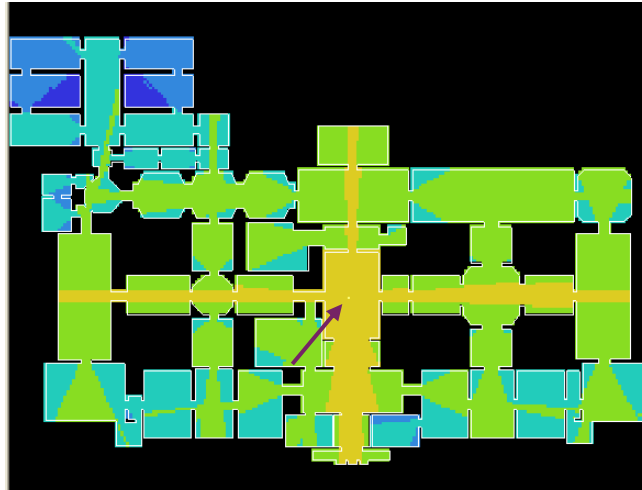
Figure 11: Step depth analysis (The arrow shows the selected location with step depth value of zero. Yellow color shows all areas with a step depth 1 value, green shows 2, light blue 3, and darker blues 4 and 5.
