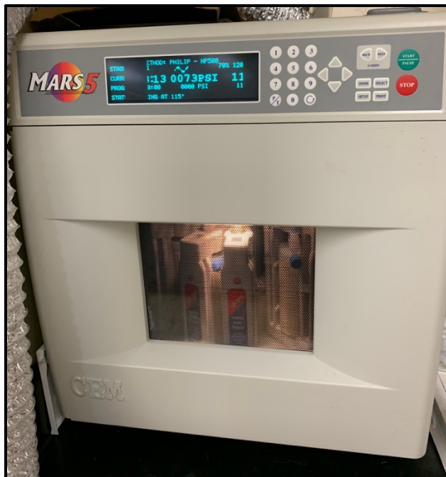
Figure 8. Photograph of Mars 5 analytical microwave digestion oven utilized for MAE.
