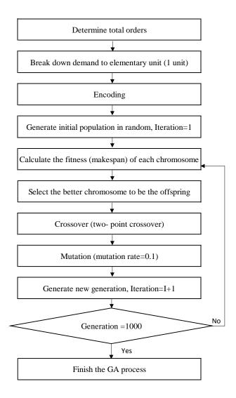
Figure 12 Flow chart of genetic algorithm procedure
