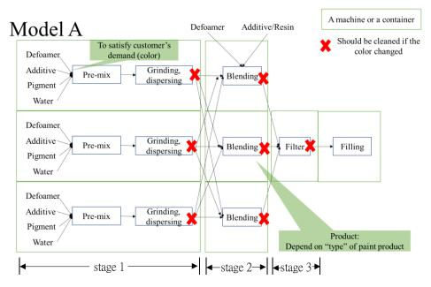
Figure 7 Illustration manufacturing process of model A
