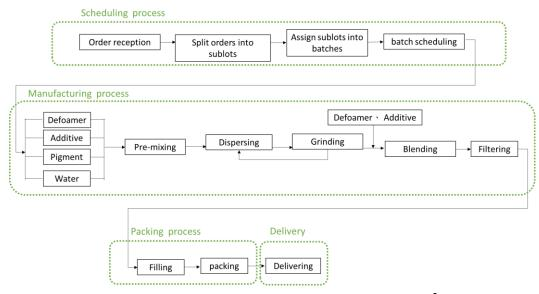
Figure 4 Overall paint production process. Source from: San Nopco<sup>5</sup>
