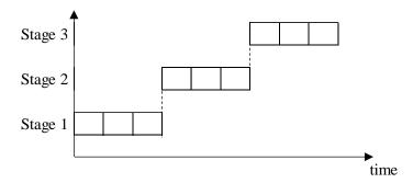
Figure 5 Process batch equals transfer batch
