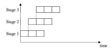
Figure 6 Process batch not equal to transfer batch
