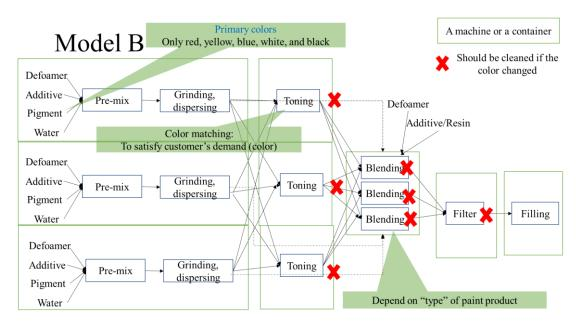
Figure 8 Illustration process of model B
