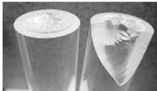
Fig.2.5 Flat and spiral fracture surface in torsion test [32].
