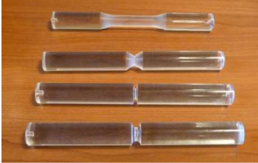
Fig.2.3 Mode III torsion testing, cylindrical testing specimen with different notches [27]
