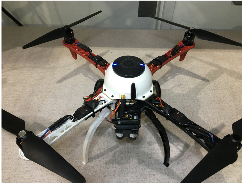
(A) Quadrotor UAV built for outdoor flights
