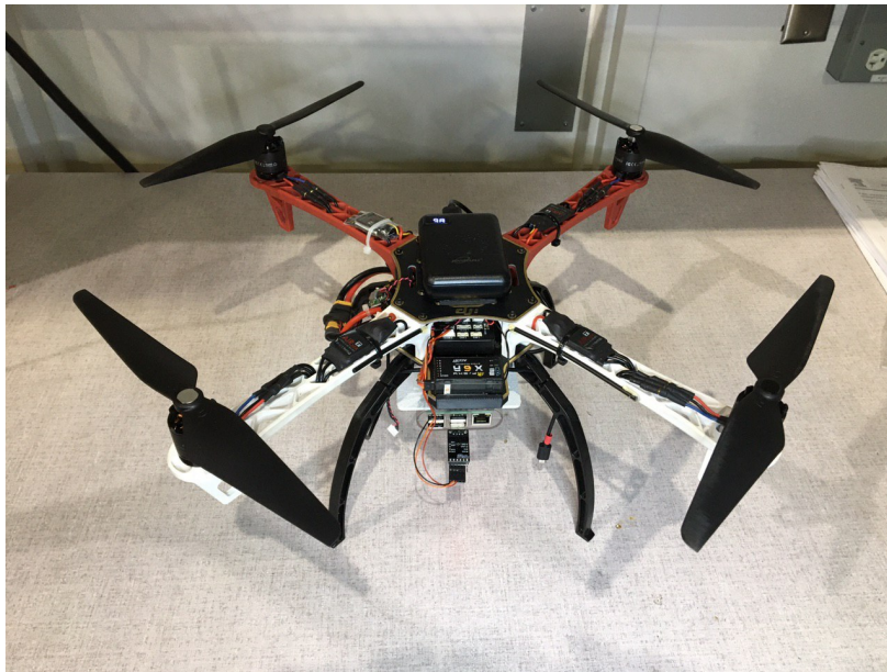
(B) Quadrotor UAV built for indoor flights
