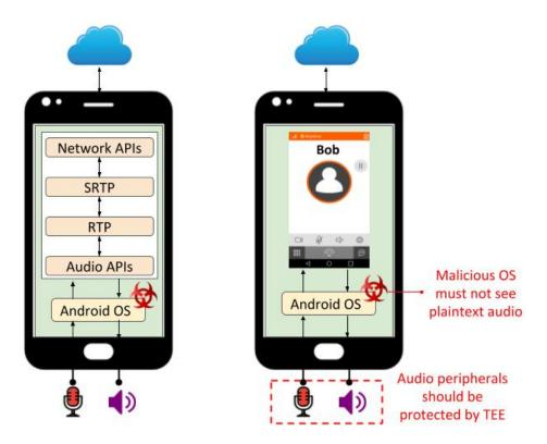
Fig. 4.2.: VoIP App Stages and Secure VoIP Requirement
