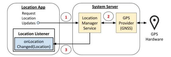
Fig. 5.13.: Default Control Flow for Getting GPS Location
