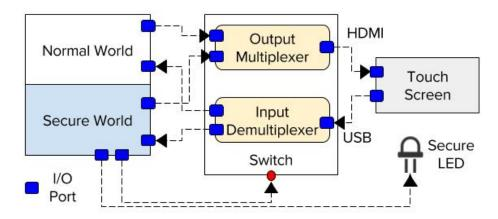
Fig. 3.12.: Hardware Setup Overview for Truz-UI
