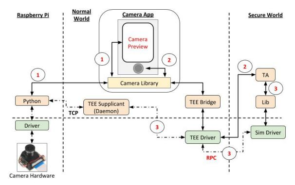
Fig. 5.11.: Truz-Sim Flow for Getting Picture from Camera
