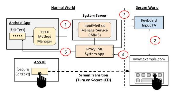
Fig. 3.4.: Seamless Keyboard Binding Across OS
