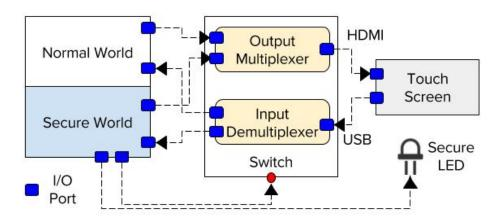
Fig. 5.17.: Hardware Setup Overview for Truz-UI (From Chapter 3)
