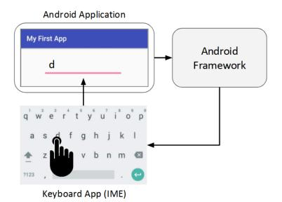
Fig. 2.3.: Android Input Method Framework Overview
