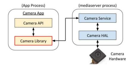
Fig. 5.10.: Default Control Flow for Getting Picture from Camera
