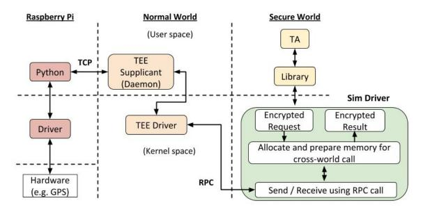
Fig. 5.8.: Use of RPC by Simulation Driver
