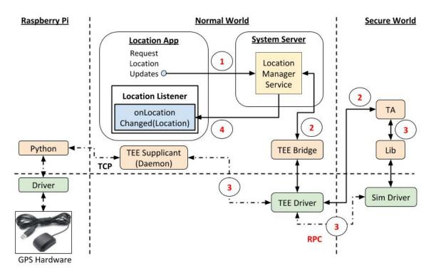
Fig. 5.14.: Truz-Sim Flow for Getting GPS Location
