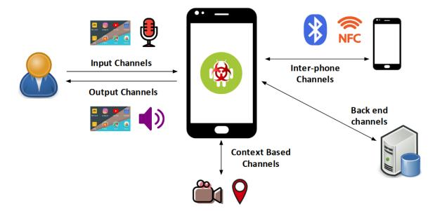
Fig. 1.1.: Smartphone Interaction Channels
