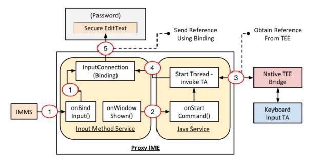
Fig. 3.7.: Proxy IME Commiting Reference Obtained from Keyboard Input TA
