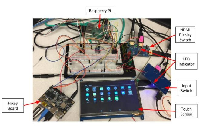
Fig. 3.13.: Hardware Test Setup for Truz-UI
