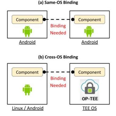
Fig. 1.4.: Types of Binding
